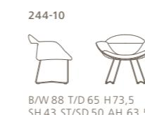
Foam-moulded seat and back with wadding and belt suspension. Steel frame, matt powder-coated black or highly polished chrome-plated.
